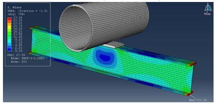
Other aspects during the development showed that the support friction between the pipe and the support beam had to be addressed. We developed a non-slide compound to ensure that the longitudinal pipe load exerted during pipe expansion and contraction did not add to excessive flange/beam rotation.
